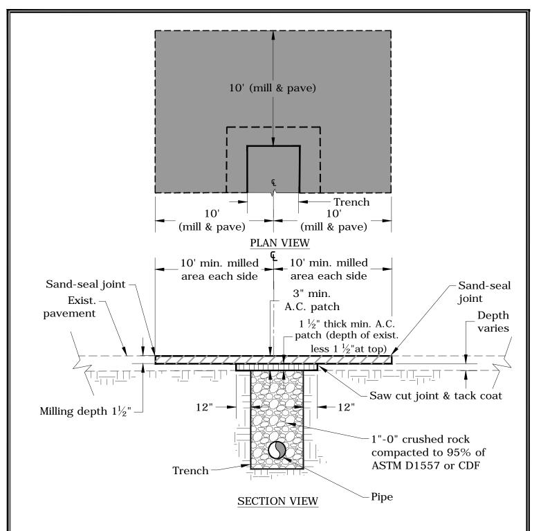
Notes: 1) The normal trench patch will be a 'T' cut as shown above. 2) If a road has been paved within the last 5 years, the trench patch shall be patched with min. 3" of A.C. after A.C. has cured, an area 10 feet on all sides will be milled 1  $\frac{1}{2}$ " and paved with a paving machine. 3) Use Class 4 backfill method (see City standard drawing S6-01). 4) Asphalt compaction will be 91% of OSHD TM 306B (rice).
