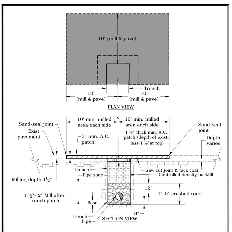
Notes: 1) If a road has been paved within the last 5 years, the trench patch shall be patched with 3" of A.C. after A.C. has cured, an area 10 feet on all sides will be milled  $1\frac{1}{2}$ " and paved with a paving machine. 2) CDF will be required on all collector and arterial streets.
