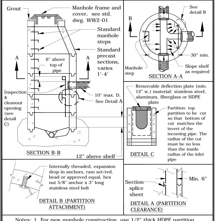
Notes: 1. For new manhole construction, use 1/2" thick HDPE partition. For retrofitting, when the cone will not be removed, use 1/4" thick hdpe partition. 2. Partition width may vary depending on manhole conditions. When retrofitting, contractor shall build to appropriate dimensions.
